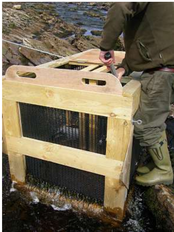
Wooden letterbox trap in use during period of low water on the River Tirry - Photo Hugh Mackenzie
